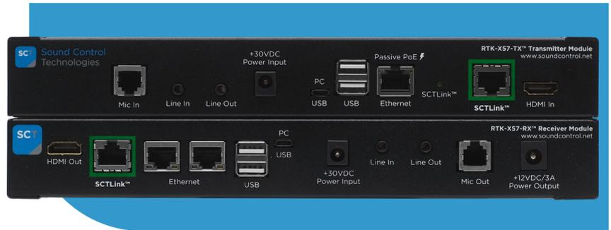
Sound Control Technologies (SCT) Table Extension Kits are designed to bring you the inputs from the Poly Studio video bar backplanes right to the *table!* The RTK-X57™ kit provides a reliable transparent link between the table devices and the connected Poly device.
