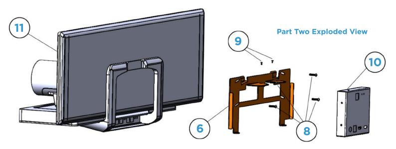
**Step 7:** Looking at the back of your Cisco SpeakerTrack 60 (No. 11, Qty 1), align Cisco's grey fabric microphone plate against the SpeakerTrack 60's vertical rear bracket; *Do not use Cisco's provided Torx screws for this step*.
