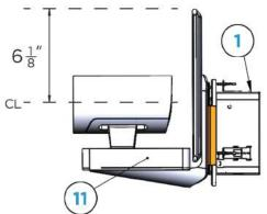
**Step 4:** Check that the Wall Clamp (No. 2) flange is in the retracted position. Place the flange through the knockout hole and tighten in place, turning clockwise; *Do not over tighten!*
