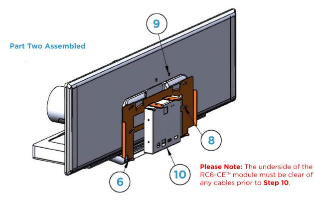
Step 10: Hang Part Two Camera Assembly on Part One Wall Box Assembly.
