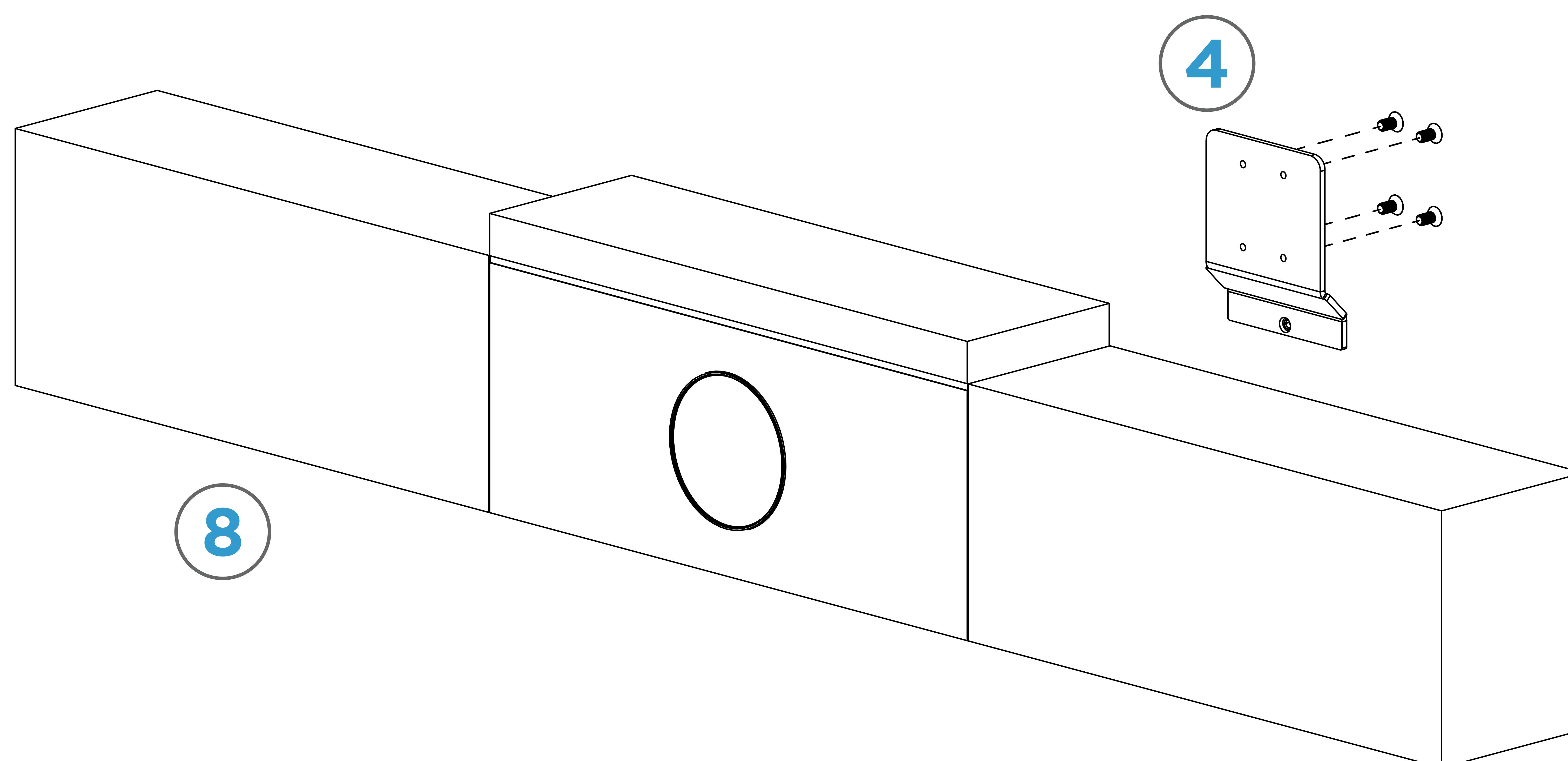
**STEP 6:** Slide camera assembly into slot of Adapter Plate and secure with 6-32 x 1/4" Phillips screw (No. 7, Qty 1). Then slide Cubby Face Plate top (No. 6, Qty 1) down onto tabs in Cubby Backbox.
