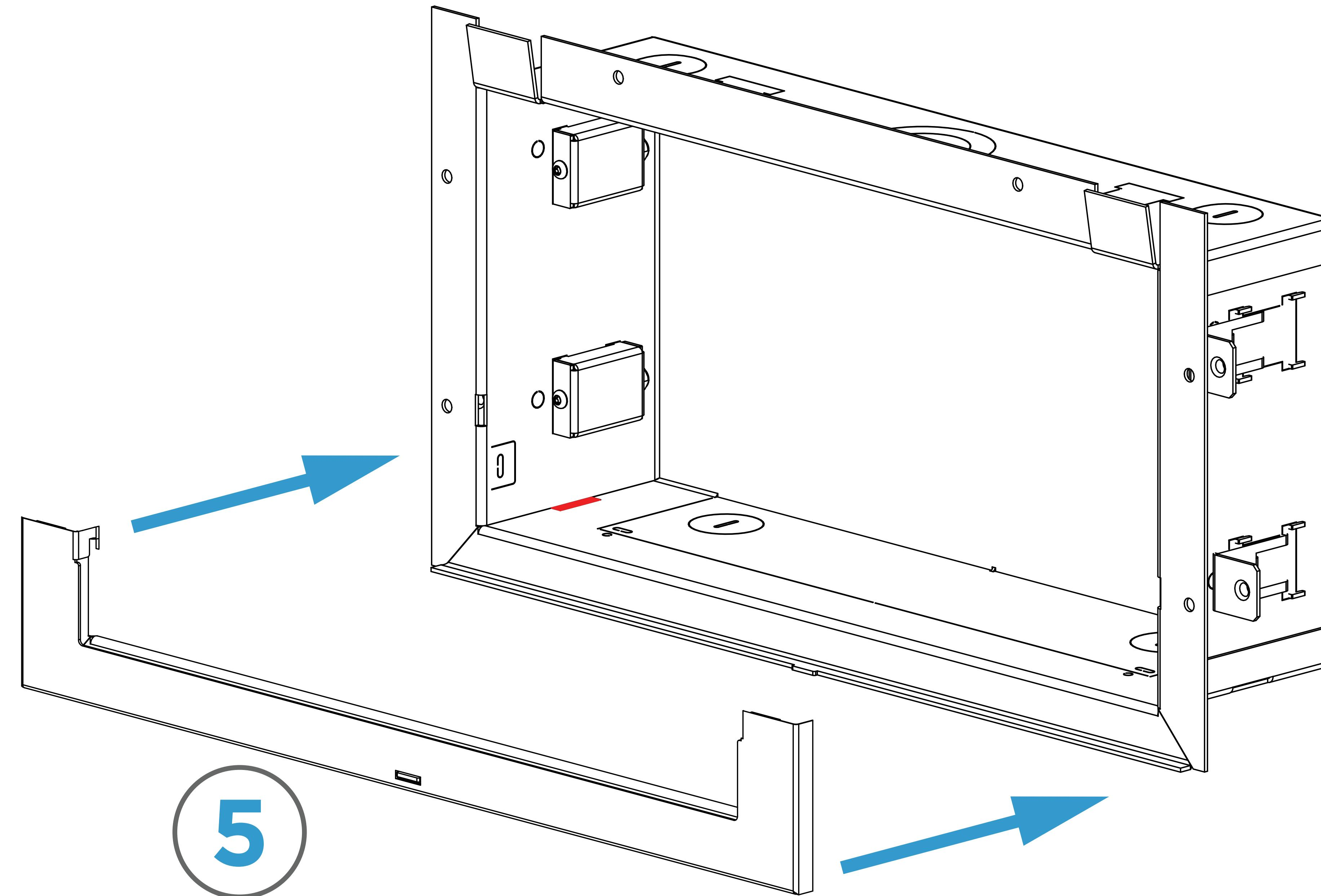
**STEP 4:** Slide Camera Plate (No. 3, Qty 1) down into Cubby slots (shown in red) and push forward to engage. Then pry tabs inward to lock Camera Plate in place.
