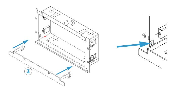
**STEP 4:** Set VB1/adapter plate assembly into camera plate slots and tighten securely from underneath.
