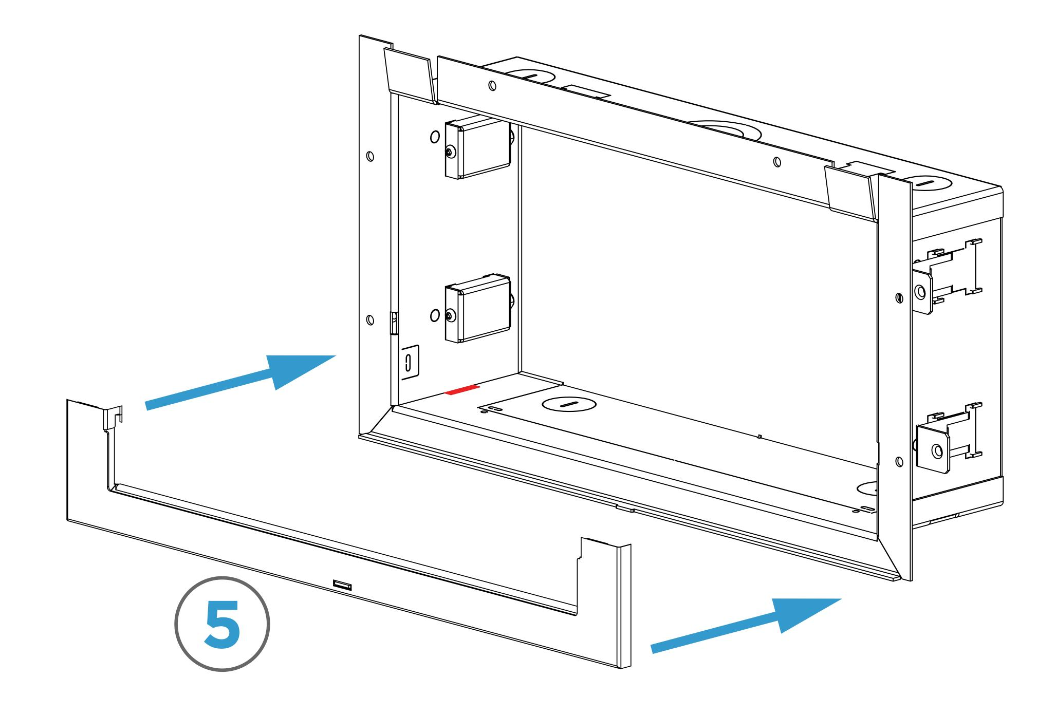
**STEP 3:** Slide Camera Plate (No. 3, Qty 1) down into Cubby slots (shown in red) and push forward to engage. Then pry tabs inward to lock Camera Plate in place.
