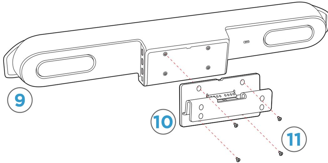
**STEP 4:** Partially install 6-32 x 1/4" White Slotted Screws (No. 7, Qty 2) into Adapter Plate (No. 4, Qty 1) using the front holes. Do not tighten. Slide Adapter Plate into Poly Hinge Bracket and secure with M5 x 8mm Philips Flat Head Screws (No. 8, Qty 4).
