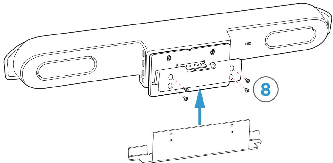
**STEP 5:** Slide camera assembly into slots on Camera Plate and tighten screws from bottom.
