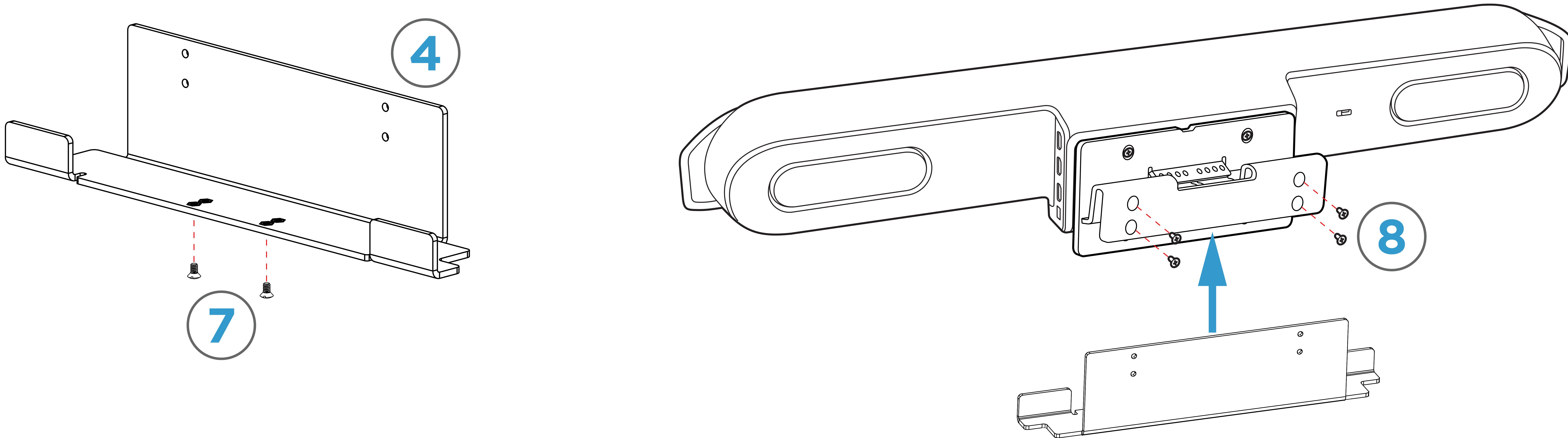
**STEP 5:** Slide camera assembly into slots on Camera Plate and tighten screws from bottom.
