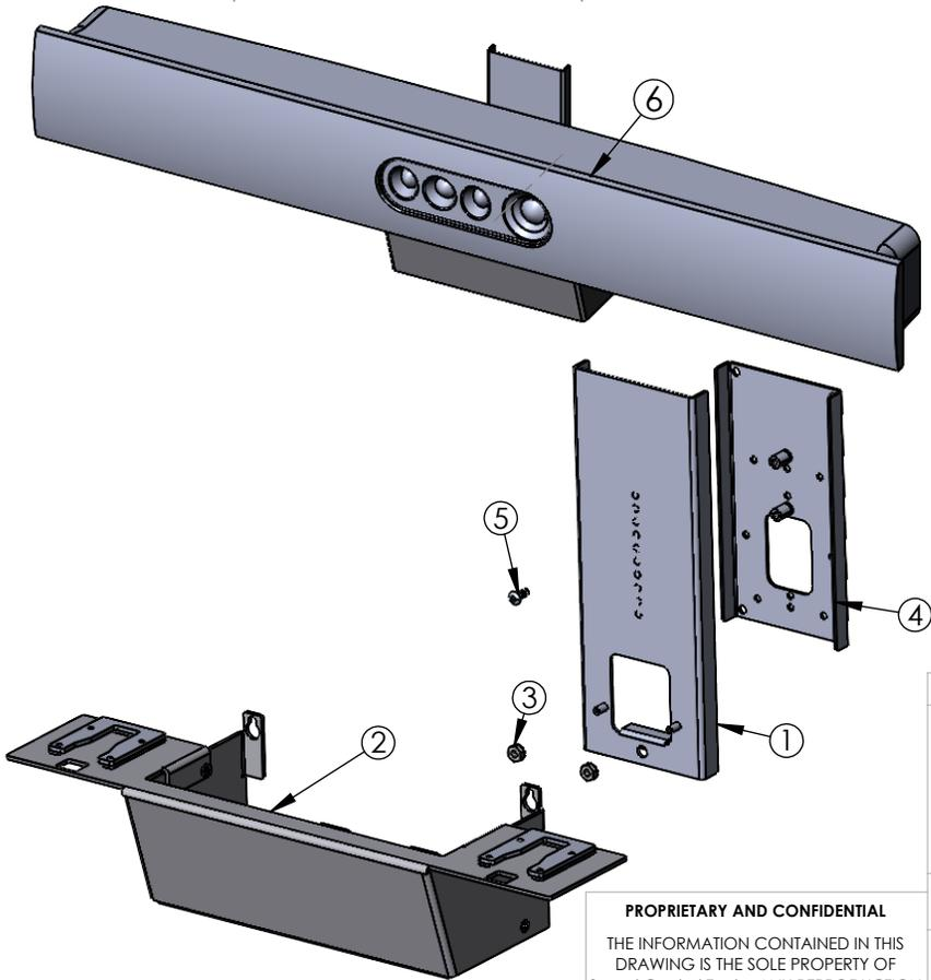
Item #4 Should be mounted to wall with Wall Anchors appropriate for the wall material.
