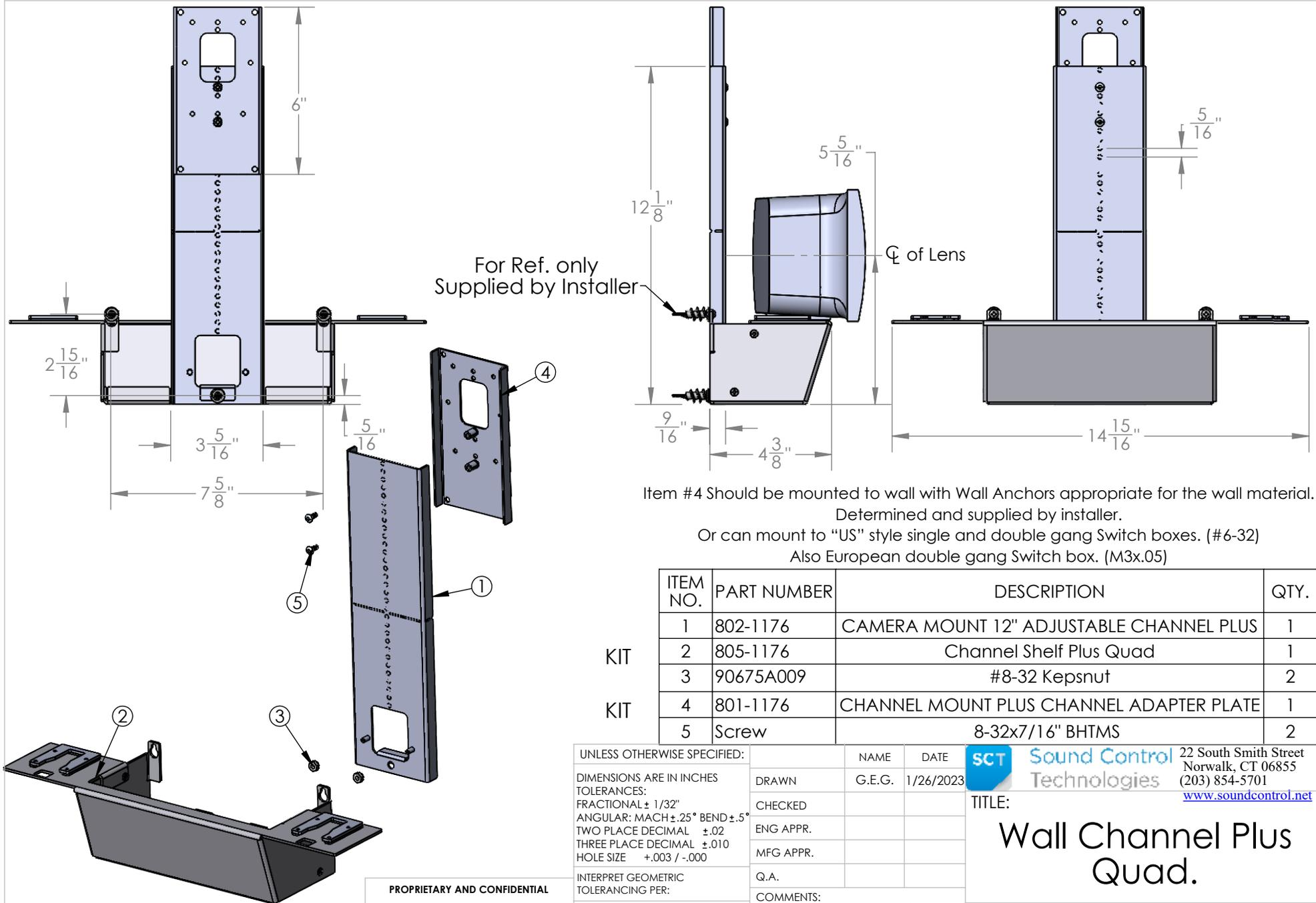
Item #4 should be mounted to wall with Wall Anchors appropriate for the wall material. Determined and supplied by installer.
