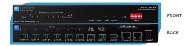
The MDC6 is a serial hub device controller designed to aggregate communications from multiple SCT devices into a single codec data connection. It features RS-232 ports to connect up to 6 supported SCT devices, and can communicate natively to supported codecs over RS-232 or IP links.
