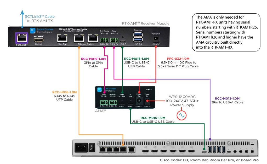
Note: DIP switch position 1 on the Receiver must be in the on position to enable Cisco communications.
